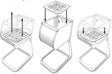
Note: when inserting the baffle plate ensure that it is pushed firmly into place and secured underneath the channel protrusions on each side of the dispenser.
