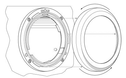
Install the appropriate baffle (see step 2) onto the ring by lining up the posts in the ring with the holes in the baffle. Be sure the baffle is completely flush with the underside of the ring and that it is inserted underneath the three retention tabs.
