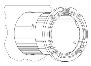
Drill four 9/64" pilot holes in the locations shown below. Fasten the dispenser with the four #10 screws provided.
