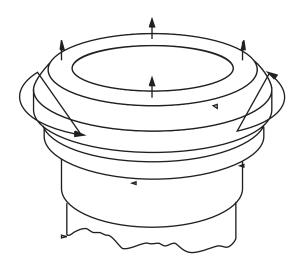
Insert the dispenser into the mounting hole. Align the "UP" mark to the top in a horizontal or angled application and to the rear in a vertical mounting application.
