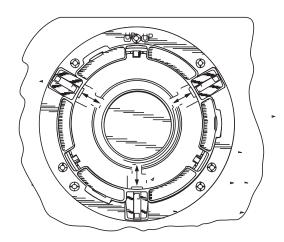
TEST: Make sure only ONE cup dispenses at a time. If more than one cup is being dispensed at a time move adjustment clips inward. If cups are difficult to dispense move adjustment clips outward.
